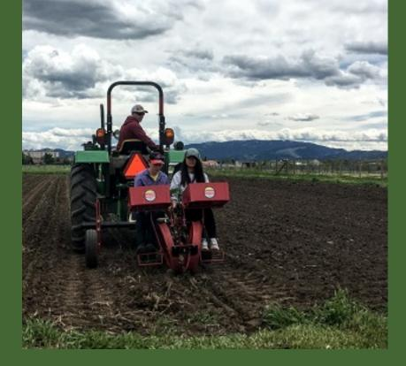
The transplanter is a tractor-operated implement that saves time, money and labor. The transplanter is a 3-person operation – a tractor driver and two others working the machine. Plants started from seed in a greenhouse weeks prior, are brought to the field as seedlings where they are planted. Because of our long, cold springs here in Montana transplanting is absolutely necessary.
