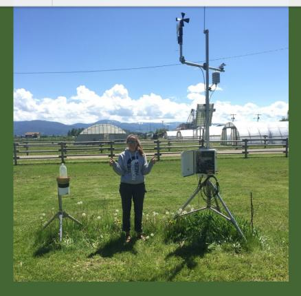
Thanks to funding from MSU's College of Agriculture, MSU's Horticulture Farm has its own weather station. The weather station measures temperature, relative humidity, wind speed and direction, barometric pressure, sunlight intensity, and rainfall. Conditions are averaged hourly and reported on <a href="this website">this website</a> via a cellular modem link.
